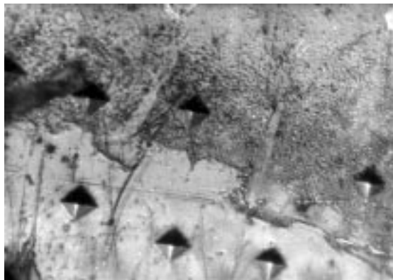
Fig. 1. Stripe of fine precipitates on the slanting microsection of the specimen doped by gold with the imprints of the indenter
